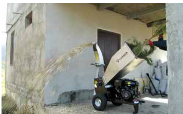
Fig. 6: Mulching machine preparing mulch from sanitary cutting residues
